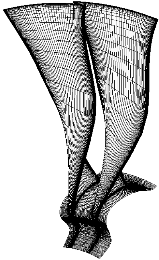
Fig. 6 Blade geometry and surface mesh of the three-dimensional fan.
